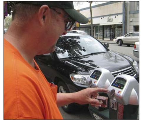
Karlan Larson of Traffic Operations tests a new solar-powered meters. The new meters accept credit cards in addition to coins.
